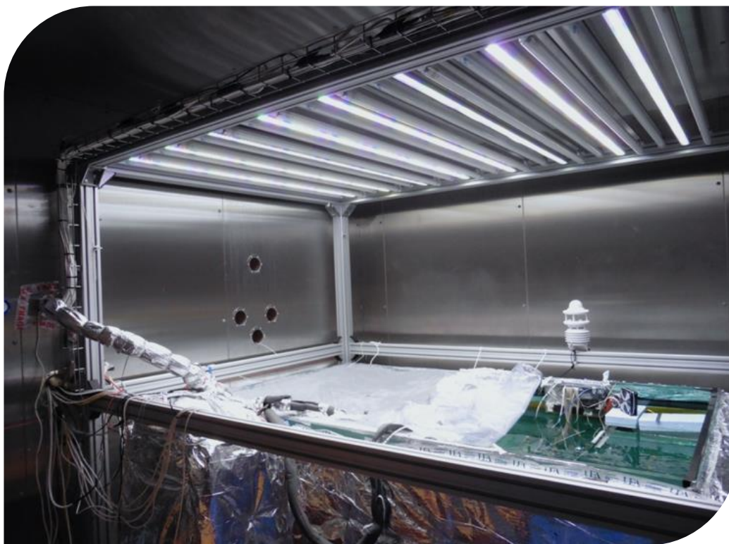
Figure 6: The sea-ice chamber under visible light illumination. In this instance, a polytetrafluoroethylene-fluorinated ethylene propylene atmosphere is partly enclosing the tank which measures 2.4 m x 1.4 m x 1.1 m and contains ~3,500 litres of sea-water saturated with methane. © James Lawrence France.
